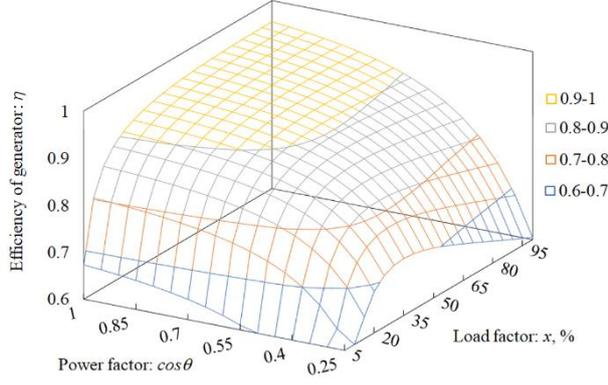
Fig 1. Efficiency map estimated by the energy dissipation mechanism of synchronous generator
