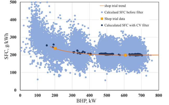
Fig 2. Shop trial data and calculated SFC data with CV value less than 0.01 for 10min.
